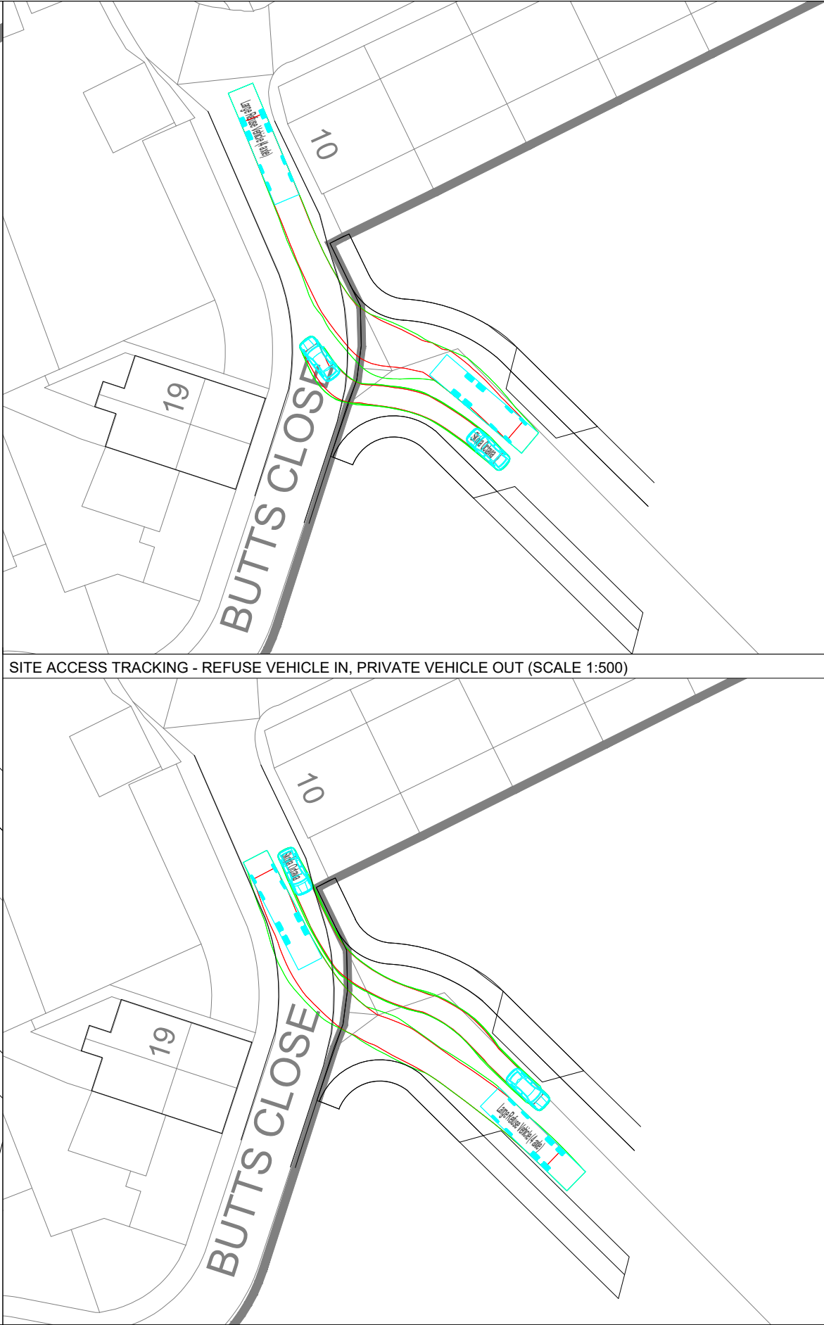
SITE ACCESS TRACKING - REFUSE VEHICLE OUT, PRIVATE VEHICLE IN (SCALE 1:500)
